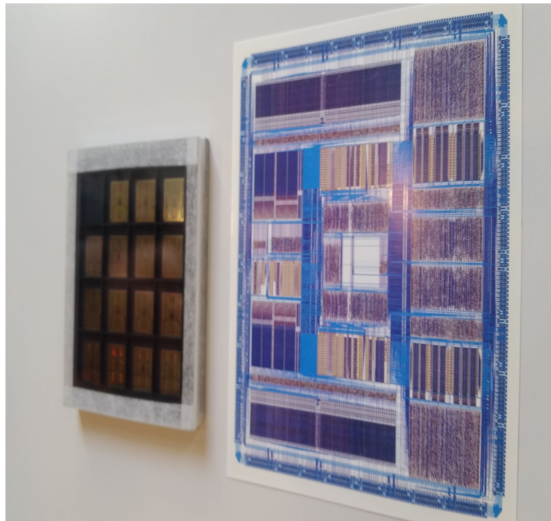
Figure 4.4: Picture of an open hardware SoC schematics and prototype from the ALSOC team at LiP6, provided by Marie-Minerve Louërat.
